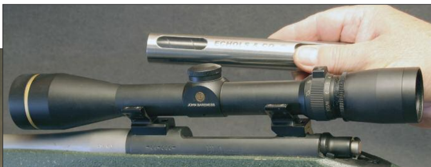
Left, the Echols mounting bar allows base screws to be tightened while the rings are perfectly aligned with each other, avoiding any misalignment. Above, once the rings are tightened to the action, the bar is removed and the scope mounted.
