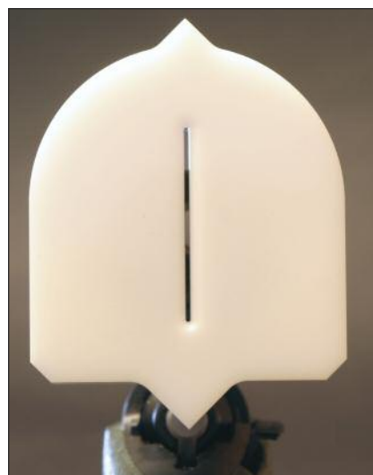
The Reticle-Tru fits over the rear bell of the scope, with the point at the bottom of the tool centered on the rear of the bolt.
